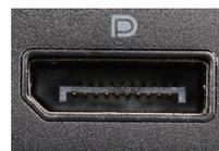
HP computers use their proprietary DisplayPort connection (small image) and is common at Taylor. The clipped corner helps distinguish it from HDMI.
