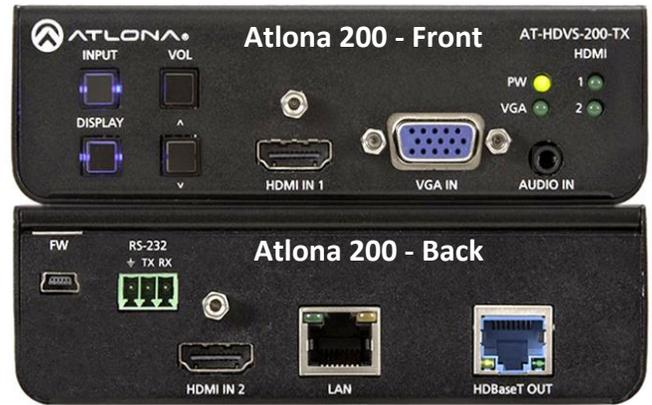
Except for the CAT cable output (HD Video Out or HDBaseT Out) on the back, none of the other connectors are used during normal operation.
